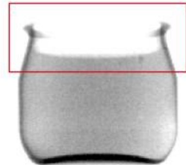
Fill level control in a yogurt cup
