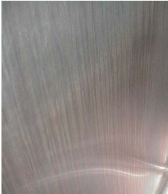
After Pre-Rinsing, Protein Film Remaining on a Food Contact Surface
