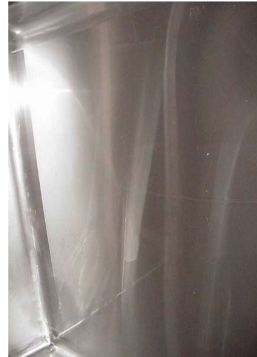
After Cleaning with a Chlorinated Detergent
